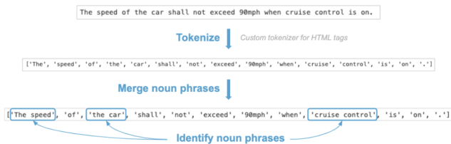
Figure 5: The text is first tokenized, then tokens are tagged with PoS labels, and finally noun-phrases are formed by merging adjacent tokens where appropriate. The noun-phrases are now considered extracted and fed into Step 2.
